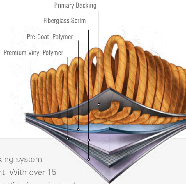
EcoFlex™ ICT is a premium vinyl modular backing system containing a minimum of 35% recycled content. With over 15 years in the marketplace, its ultra dense construction is engineered to offer superior performance while giving greater cushioning properties.
